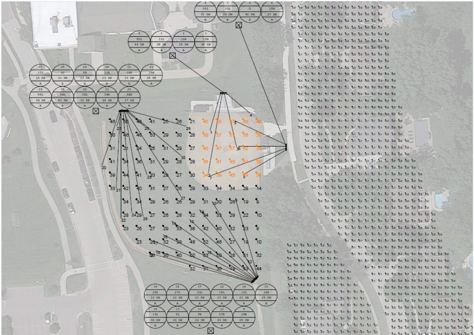
Sample photometric calculation – Baseball, 240ft, 4(65ft), Class III
